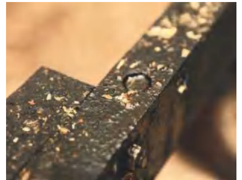
A handy drill hole for a reservoir of walnut oil for lubricating the end-grain, which turn easily in the centre rods
